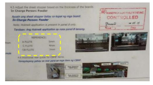
USE THE REFERENCE SIZE OF THE SHEET FOR THE SET-UP OF FEEDER AREA.
